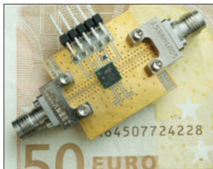
▲ Fig. 1 10 MHz to 40 GHz MIC module mounted on an application board.
